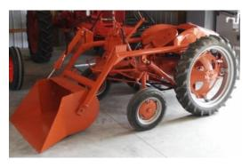
The first is a G equipped with a loader. Richard Graves brought this unique piece and said it came all the way from New Jersey where it was used to unload railcars. Its small size would certainly make working in close quarters much easier. Richard reported it can be a little "tippy" when loading on a trailer.
